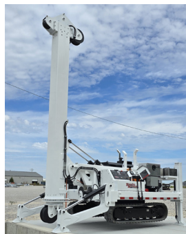
TELESCOPING MANHOLE BOOM
