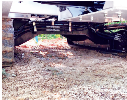
BRIDGESTONE TRACKS (TRACK WIDTH OF 79 1/2")
