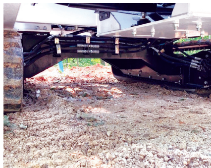
COMPACT DESIGN (TRACK WIDTH OF 79 1/2")
